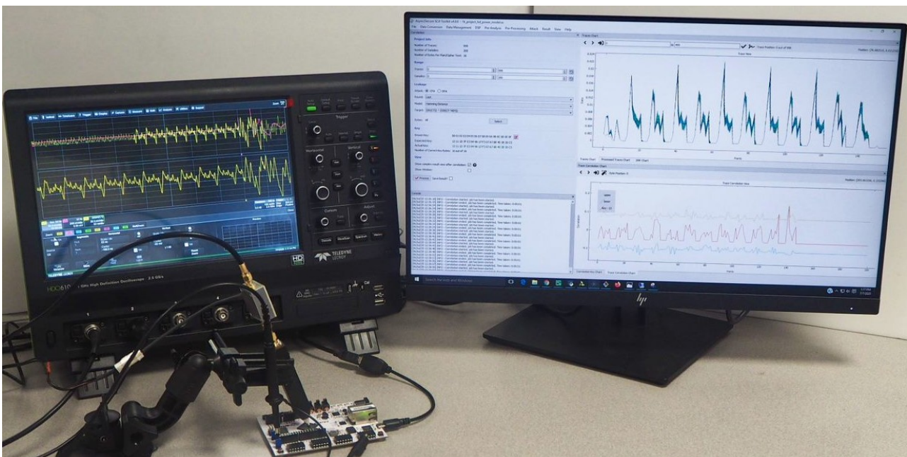
Fig. 2: An FPGA prototype SCA evaluation using our SCA evaluation platform
